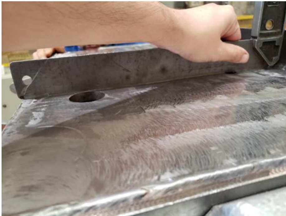
Figure 15: Verification of the levelness of the base plate
